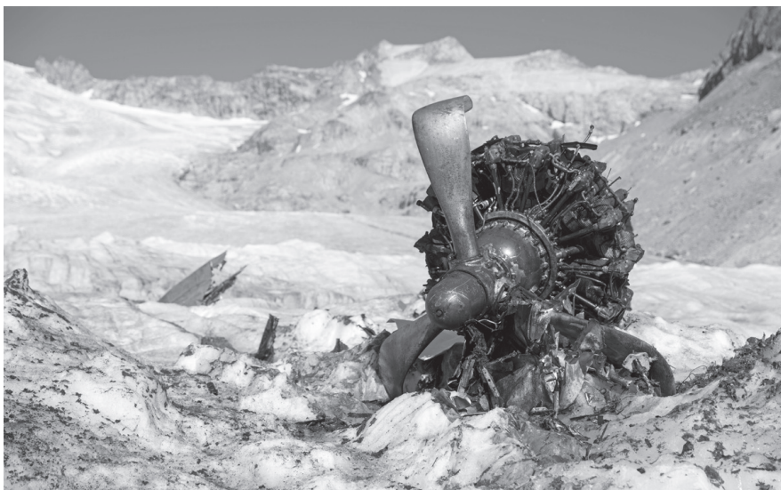
REMAINS OF A PRATT & WHITNEY R-1830 TWIN WASP ENGINE FROM THE US C-53 SKYTROOPER THAT CRASHED-LANDED ON GAULI GLACIER IN 1946
